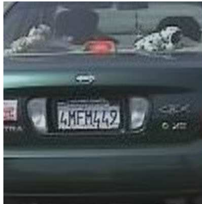
Fig. 15. License plate HR image reconstructed by the NNSR algorithm
