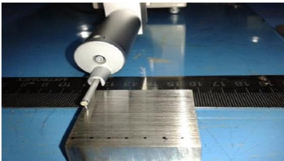
**Fig. 7.** Testing Roughness with profilometer of contact
