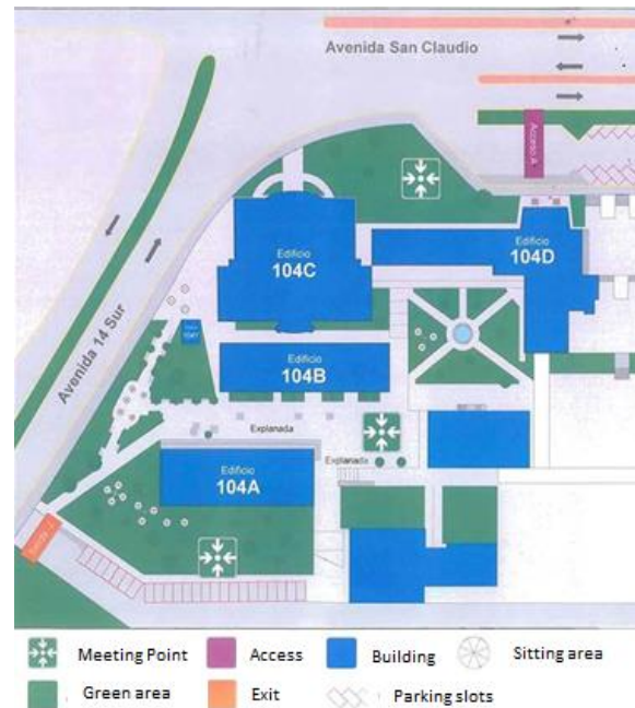
Fig. 2. 2D models of the virtual campus, Polygons drawn with Google Map Maker® exported as KLM then mapped on a HTML canvas
