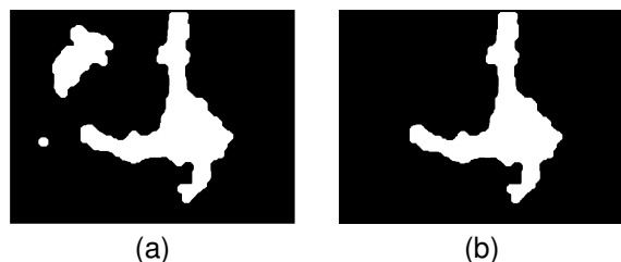
Fig. 4. a) Morphological opening and b) Filtering by area
