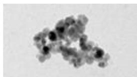
**Fig. 2.** TEM-multi-domain magnetite core [7]
