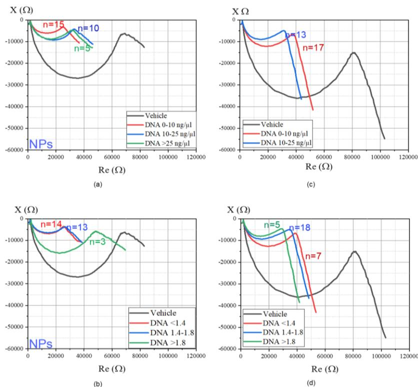
**Fig. 4.** (a) Nyquist diagram classified based on DNA concentration assisted with nanotechnology (b) Nyquist diagram classified based on DNA purity assisted with nanotechnology, (c) Nyquist diagram classified based on DNA concentration after the purification with nanotechnology (d) Nyquist diagram classified based on DNA purity after the purification with nanotechnology
