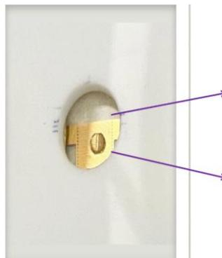
**Fig. 1.** Gold film microelectrodes
