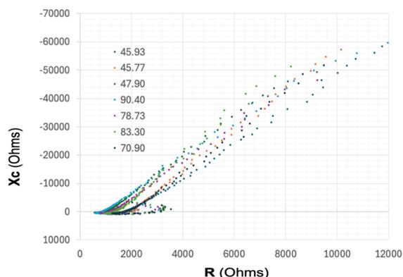
**Fig. 3.** Scatter plot Resistance (R) vs Reactance (Xc) for total DNA concentrations
