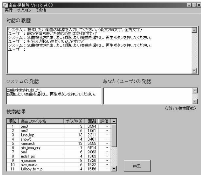
Fig. 5. A captured snapshot of the user interface for retrieval. The text box in the upper part of the screen displays dialogue history, the text box in the left-middle part displays reports and instructions from the system, the text box in the right-middle part is for the user input, and the text box in the lower part displays the results of the most recent retrieval. Rank, names of musical pieces, data size, distance, and so on are also displayed in this text box.
