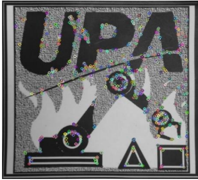
Fig. 4. Model points obtained with ORB descriptor using OpenCV 2 library
